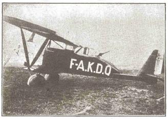
A strange craft, but a fine performer. The French Breguet two-seater reconnaissance ship, which is powered with a 650-hp. Hisso. It has a top speed of 146, fully loaded, and the unusual tail gives the gunner a wide arc of fire.
