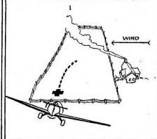
Approach it with a little excessive altitude, with the windward wing slightly down, to compensate for your drift. Let her slip just enough to keep you in line with the field.
