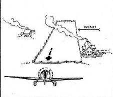
The purpose of the cross-wind landing is to get into a long, narrow field when you're forced down. We'll pick out a little cow pasture up ahead, and approach it, nosed slightly into the wind.
