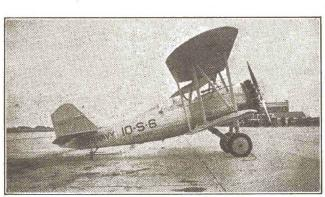
This trim craft is the Navy Vought "Corsair" O2U-4 which is used by the Navy Scouting Squadrons and thrown from cruiser catapults. A single-seater of fine performance, it carries much Navy equipment, such as deck-landing gear and flotation bags.
