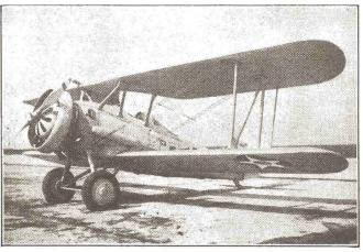
The U.S. Marine Corps goes in for smart-looking ships. This is their version of the Corsair, known as the SU-2. Note the high-caliber machine gun mounted in the upper wing, and the anti-drag ring around the motor. A two-seater beauty!
