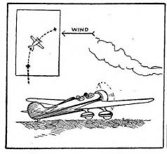
As you lose speed, gradually turn her into the wind. Remember at all times to keep the windward wing down slightly.
