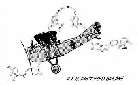
the shots were fired at little or no angle, the armor withstood the bullets up to within about 50 yards. The armor was placed to cover the two main cockpits and the lower section of the engine. Plates were also set beneath the cockpits, and there was an armored bulkhead behind the observer to protect him from attacks from the rear.
