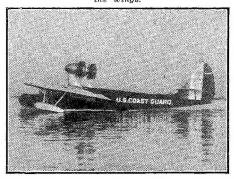
The General Aviation Flying Boat is a twin pusher. It is powered with two Pratt & Whitney "Wasp" engines, which are mounted above the wing on steel tube struts. Three-bladed Hamilton-Standard props are used. The engine nacelles are of welded steel tube construction, covered with metal and streamlined. They are interchangeable, designed to take from 400 to 600-h.p. engines.
