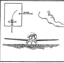
At the moment she quits flyin' and drops to the ground, kick rudder down-wind to align the wheels with the direction the ship
